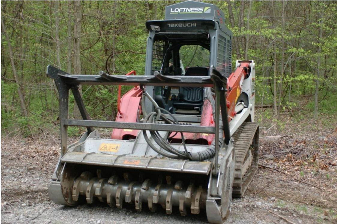
*Image 5: FirstEnergy skid steer with Fecon head used to grind vegetation*
